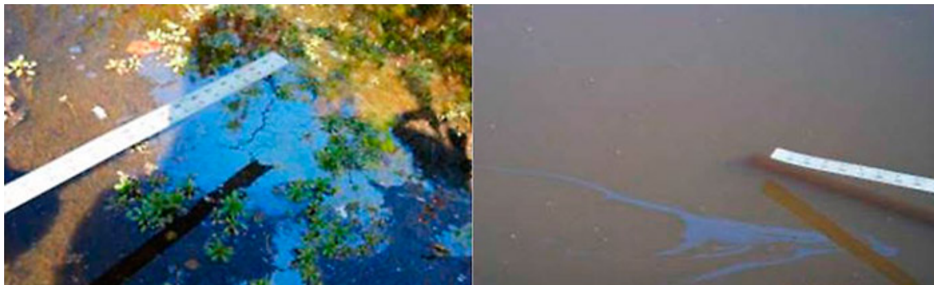
Figure S-7. Brittle sheen (left) and non-brittle sheen (right) (Stout and Uhler 2016).
